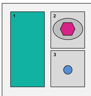
Fig 2. A schematic of a standard MRC 96-well 2-drop crystallisation plate illustrating the set-up for crystal soaking (1 = mother liquor solution, 2 = crystal to be soaked, 3 = concentrated compound).
