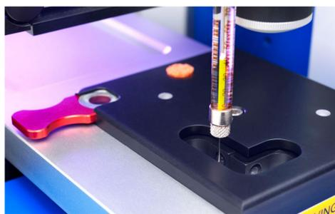
Positioning of the LCP dispense needle relative to the mosquito deck is accurate to +/- 20 µm in the X axis and +/- 5 µm in the Y and Z axes.
