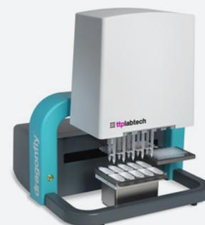
**Fig 1.** dragonfly®. The robot has a small footprint and is maintenance-free. To make a screen, the stock solutions are poured into the troughs located on the main stage (up to 10 stock solutions). Syringes are attached to the head of the robot. Once the plate is in place, the formulation protocol is selected before launching the automated making of the screen into the wells of the plate.
