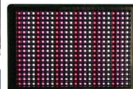
384-well source plate containing 4 step dilutions of 96 compounds
